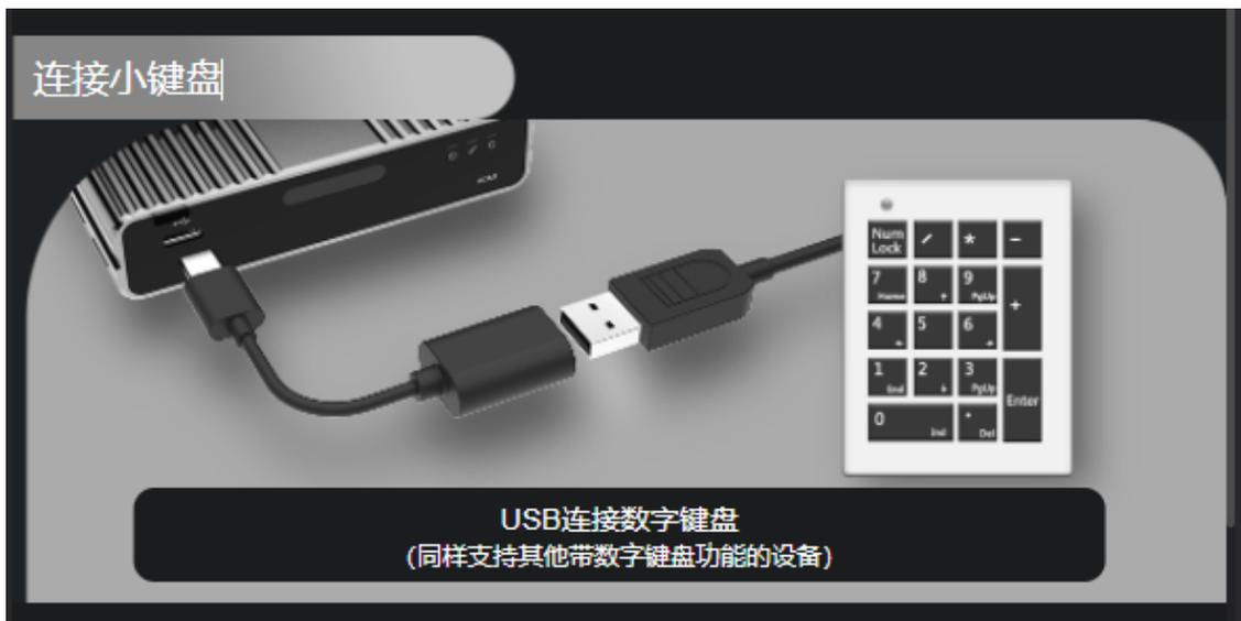
Then open the [Numlock] key on the keyboard, the light is on to indicate normal connection, and the switching operation can be performed. Select the decoding preset corresponding to 1-9 by switching the numeric keys, and 0 selects Blank.
