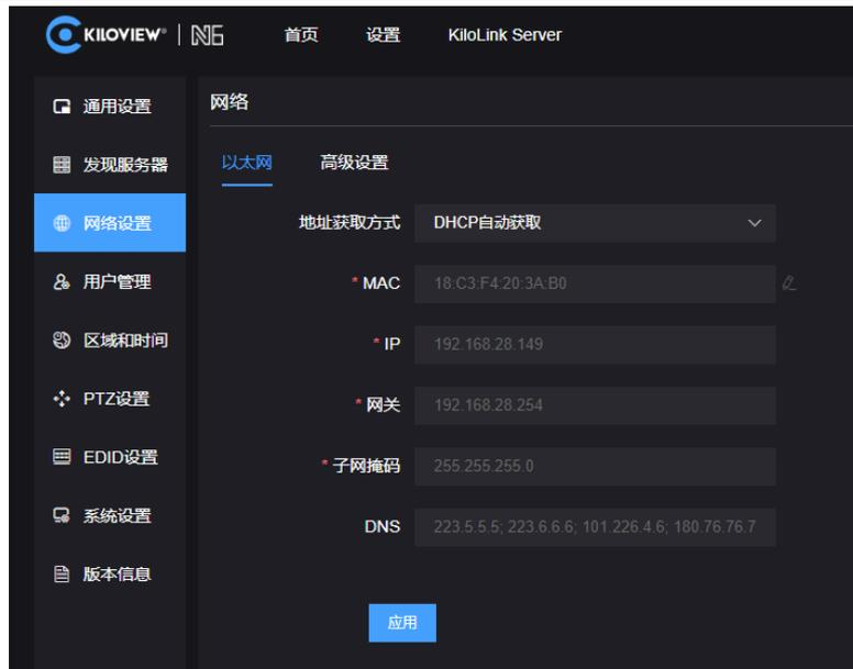
Ethernet has two types of address acquisition, one is DHCP dynamic IP and the other is static IP address.
