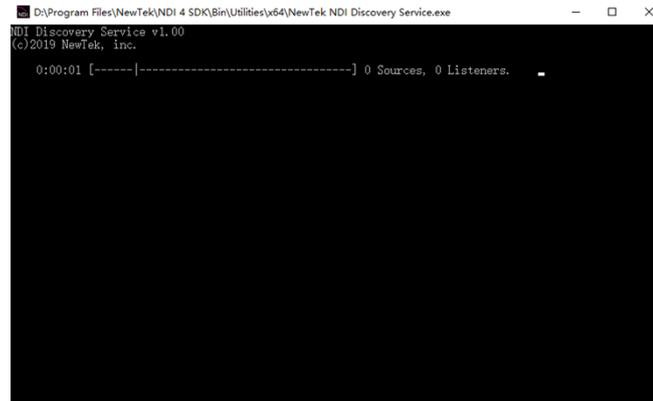
The NDI encoder configures the IP address of the receiving end in the discovery server, and the NDI will be registered to the server. It is recommended that the receiver side address be configured as a static IP address to prevent the loss of NDI connections due to IP reassignment.
